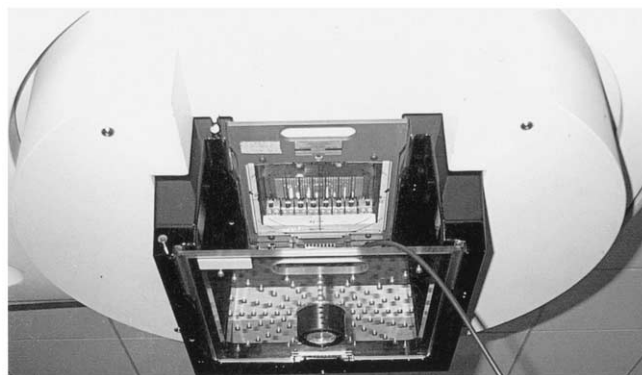
Fig. 2. The ultrasound probe plate in the accessory tray of the Siemens Primus Linac.
