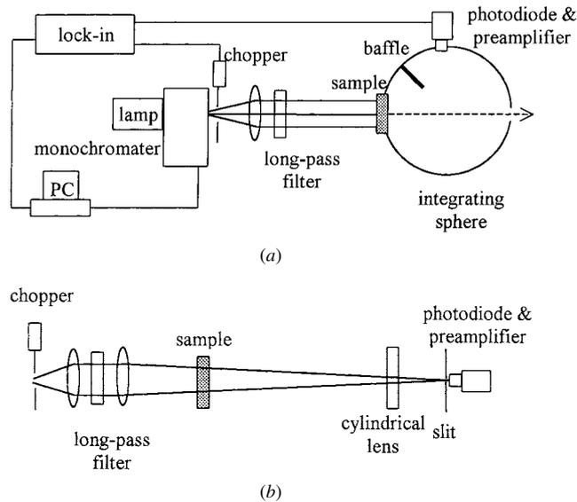
**Figure 1.** (a) The integrating sphere setup for measurements of the diffuse transmission  $T_d$ . (b) The spatial filtering set-up for measurements of the collimated transmission  $T_c$ .
