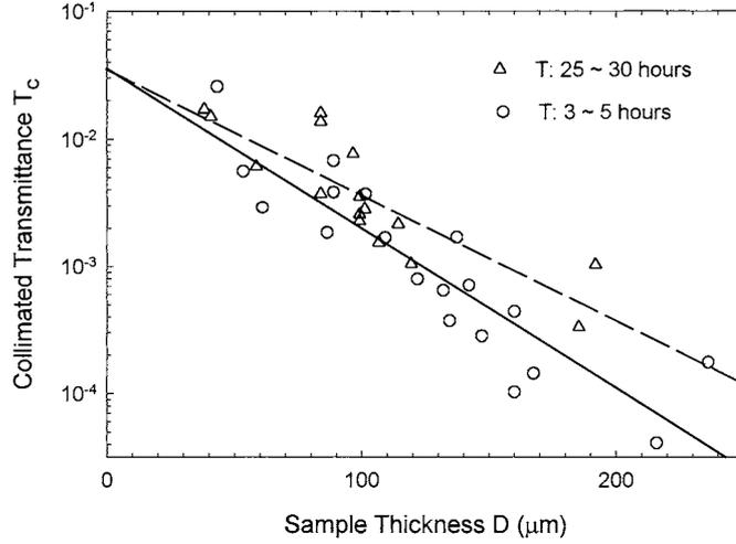
**Figure 2.** The collimated transmittance  $T_c$  of 36 samples versus the sample thickness  $D$  at wavelength  $\lambda = 980$  nm. The samples are separated into two groups with post-mortem time  $3 < T < 5$  h or  $25 < T < 30$  h for fitting with the full/broken lines to obtain two different values of the attenuation coefficient  $\mu_t$  from the slope of the lines.
