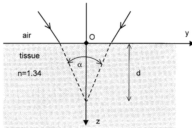
Fig. 1. Geometric configuration of a converging laser beam incident on a phantom of the biological tissue from air where  $\alpha = 30^\circ$ ,  $d = 1.0$  mm, and the refractive index of the tissue  $n = 1.34$ .
