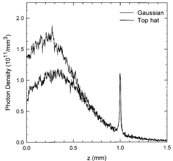
Fig. 4. Comparison of the photon density on the  $z$  axis for the two cases shown in Figs. 2 and 3.
