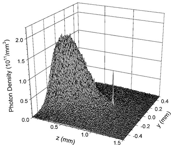
Fig. 2. Steady-state distribution of photon density in the  $y$ - $z$  plane of the tissue for a converging incident laser beam. The profile of the incident laser beam at the air-tissue boundary is Gaussian with a radius  $r = 0.268$  mm defined at  $(1/e^2)$  of the central peak. Parameters for the tissue are  $\mu_s = 10.0$  ( $\text{mm}^{-1}$ ),  $\mu_a = 0.5$  ( $\text{mm}^{-1}$ ), and  $g = 0.9$ .
