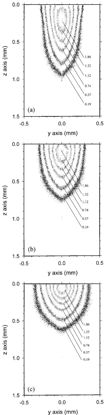
Fig. 5. Dependence of photon density on the asymmetry parameter  $g$ : (a) contour diagram of Fig. 2 where  $g = 0.9$ ; (b) same as part (a), except  $g = 0.8$ ; (c) same as part (a), except  $g = 0.6$ . The photon density of each contour is indicated by the attached number with a standard deviation of  $\pm 0.3$  in the unit of  $(10^{11}/\text{mm}^3)$ .
